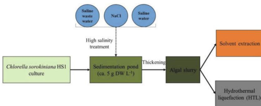
**Fig. 1.** A schematic diagram of applying high-salinity stress to the sedimentation pond of industrial algal cultivation system for high lipid induction.
