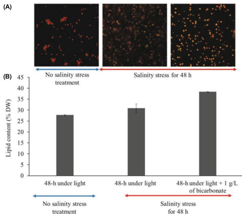
**Fig. 3.** Fluorescence microscopic images of the concentrated culture of *Chlorella sorokiniana* HS1 at the density of 5 g DW/L after 48 h under identical light and temperature conditions as the initial biomass growth phase with and without supplemental sodium bicarbonate (A), and the lipid content of harvested algal biomass with 95% confidence interval for the mean (B). 60 g/L of NaCl was applied to all salinity stress treatments for 48 h.
