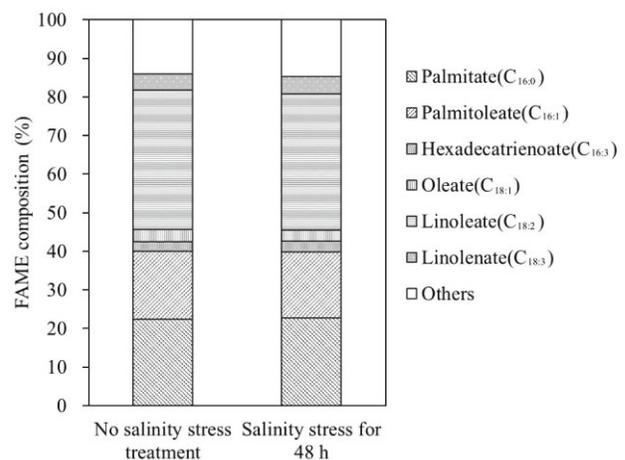
**Fig. 5.** FAME composition of *Chlorella sorokiniana* HS1 with salinity stress treatment for 48 h with 60 g/L of NaCl and 1 g/L of sodium bicarbonate and the 9-day-old culture of *C. sorokiniana* HS1 without salinity stress treatment under continuous external CO<sub>2</sub> supplementation.
